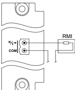
**Figure 4.74** Connection of a 2-wire resistance measurement input (RMI)
