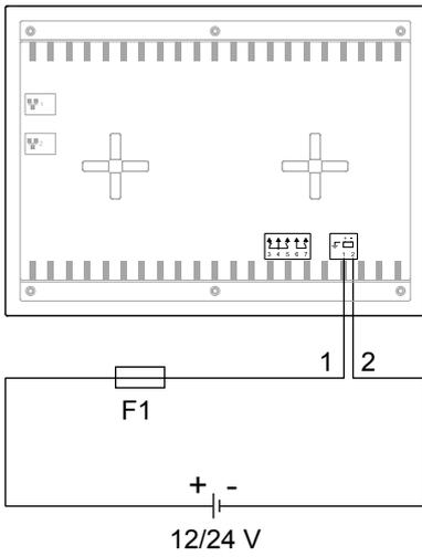
**Figure 4.97** Incorrect wiring of the power supply
