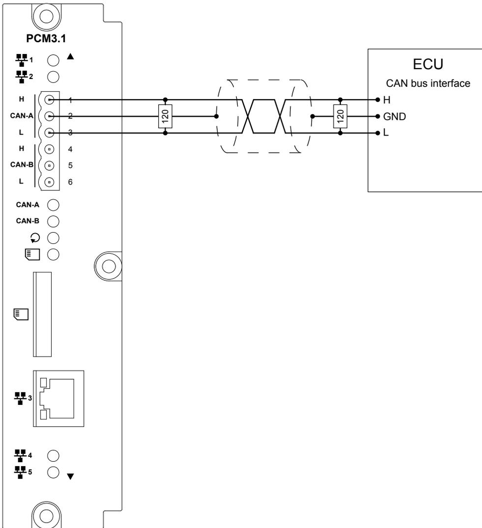
Use 120 Ω (Ohm) shielded twisted pair cable. Terminating resistors at the ends of the cable must be 120 Ω (Ohm).
