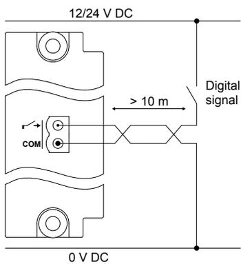
**Figure 4.25** Example: Shielded wire for compliance with EN60255-26
