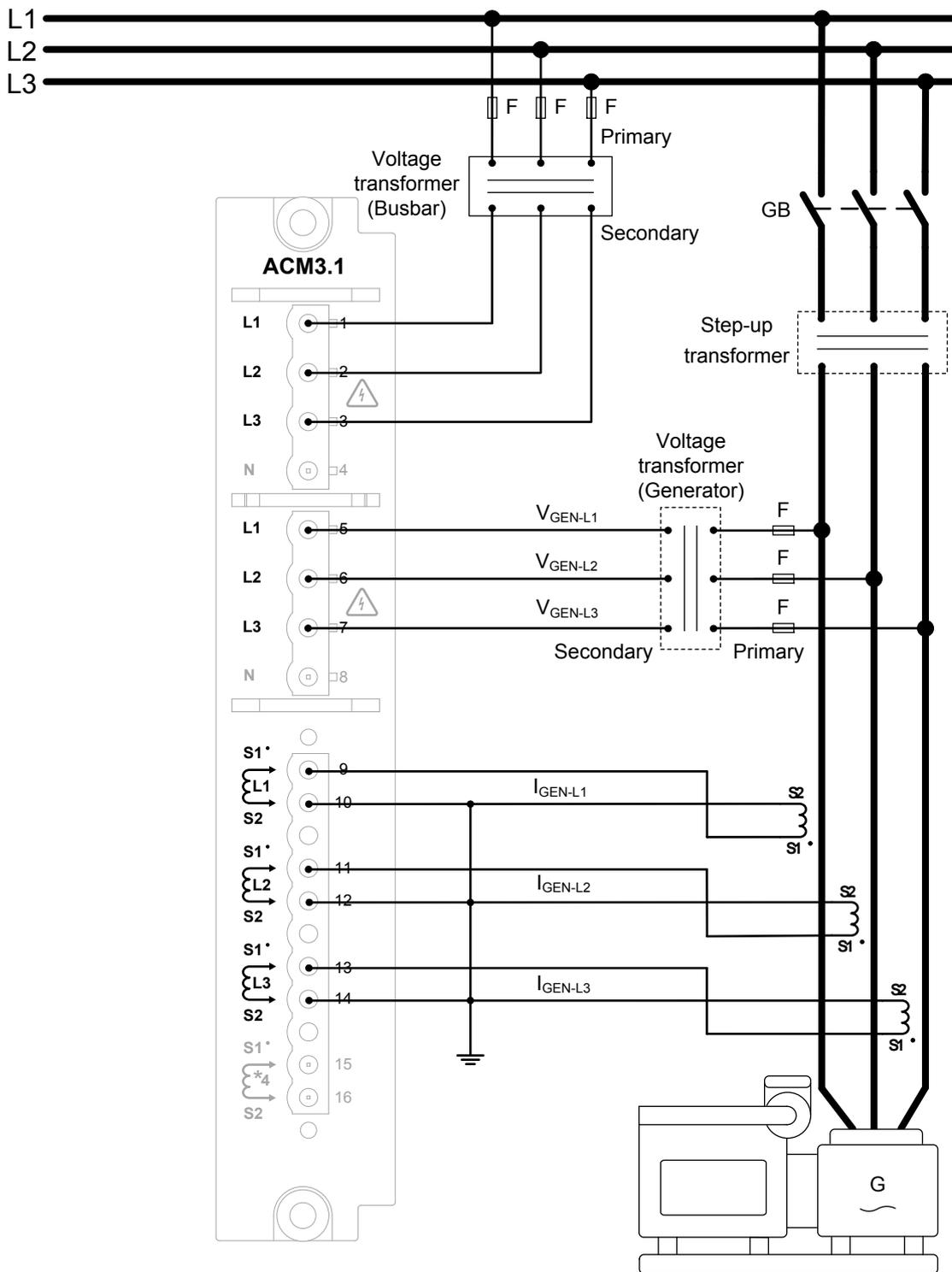
The example shows grounding on the S2 side of the current transformers. You can choose to ground the S1 side of the current transformers instead.
