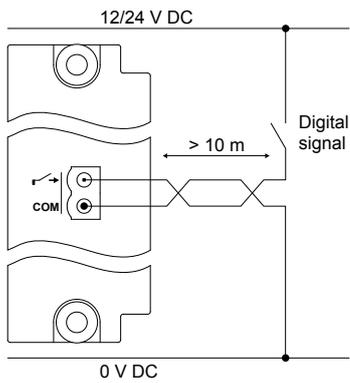
**Figure 4.17** Example: Shielded wire for compliance with EN60255-26
