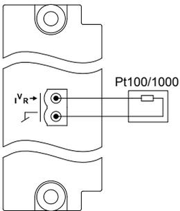
**Figure 4.32** Connection of a 3-wire Pt100/1000 sensor
