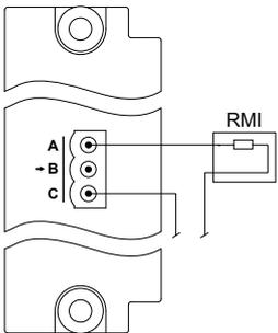
**Figure 4.44** Connection of a 2-wire resistance measurement input (RMI)
