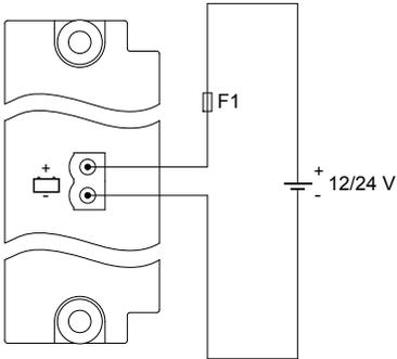
**Figure 4.78** Incorrect wiring of the power supply
