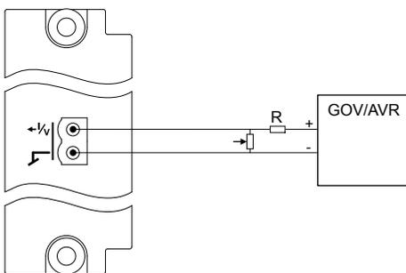
Typical value for the resistor is 2.5 kΩ, while the potentiometer is 5 kΩ.
