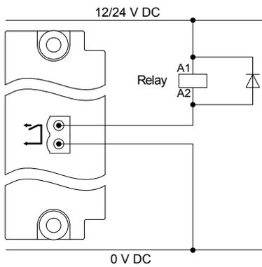
Install a freewheeling diode (
