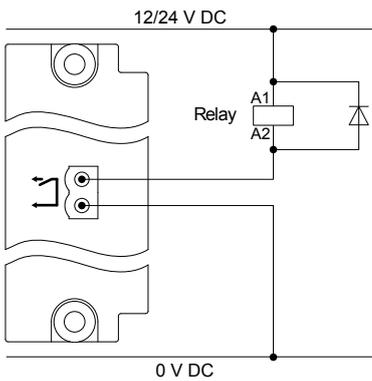
Install a freewheeling diode (
