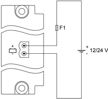
**Figure 4.7** Incorrect wiring of the power supply
