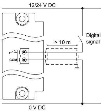
**Figure 4.87** Example: Closed contact for compliance with EN60255-26
