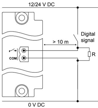
**Figure 4.16** Example: Twisted wire for compliance with EN60255-26
