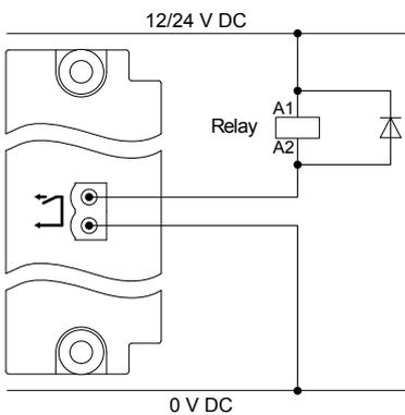
Install a freewheeling diode (
