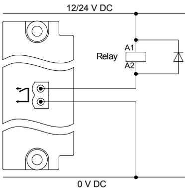
Install a freewheeling diode (
