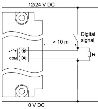
**Figure 4.65** Example: Twisted wire for compliance with EN60255-26
