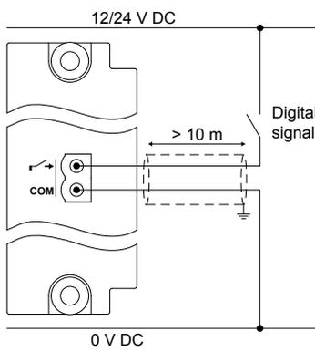
**Figure 4.55** Example: Closed contact for compliance with EN60255-26
