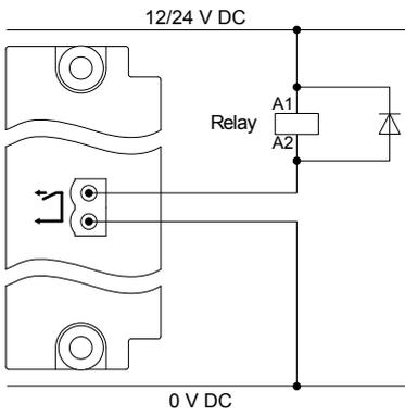
Install a freewheeling diode (
