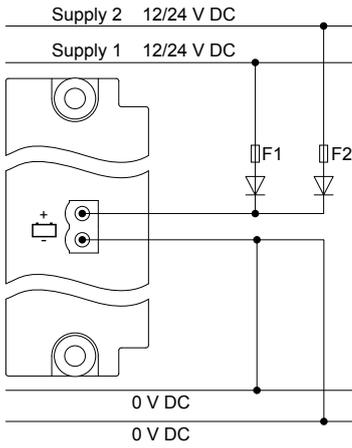
We recommend a 2 A slow blow fuse for F1 and F2, and that the diodes are rated 50 V or higher.
