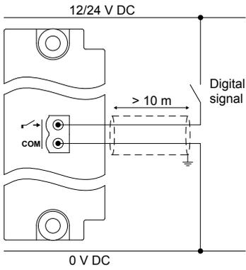
**Figure 4.26** Example: Closed contact for compliance with EN60255-26
