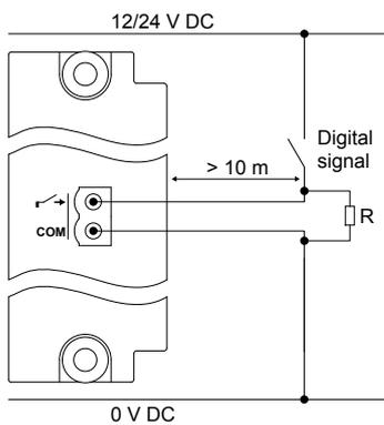
**Figure 4.85** Example: Twisted wire for compliance with EN60255-26
