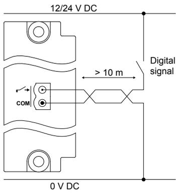
**Figure 4.86** Example: Shielded wire for compliance with EN60255-26
