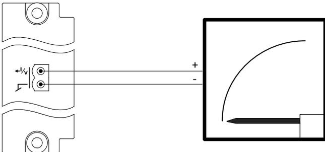
We recommend you use instruments from the DEIF DQ moving coil instrument series. See <http://www.deif.com> for more information.
