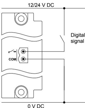
**Figure 4.49** Example: Digital input wiring (common = 12 or 24 V)
