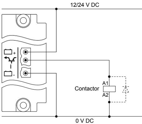
**NOTE** You can install a diode (
