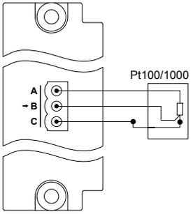
**Figure 4.42** Connection of a 4-wire Pt100/1000 sensor
