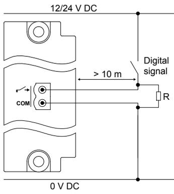
**Figure 4.53** Example: Twisted wire for compliance with EN60255-26
