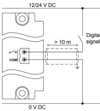
**Figure 4.67** Example: Closed contact for compliance with EN60255-26
