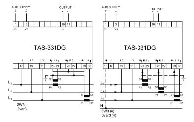
It is not necessary to protect the measuring voltage inputs. But it is recommended to use a 2A fuse for the supply input (terminals 1 and 3).
