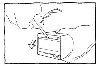
The front panel is removed by means of a screwdriver. The front panel may be loosened in the right side first and is then totally demounted by moving the screwdriver towards left.
