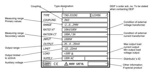
The un-configured transducer is provided with a label with the following data:
