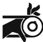
Carefully rotate the alternator toward the cylinder block while loosening the V-belt. Failure to comply may result in minor or moderate injury.
