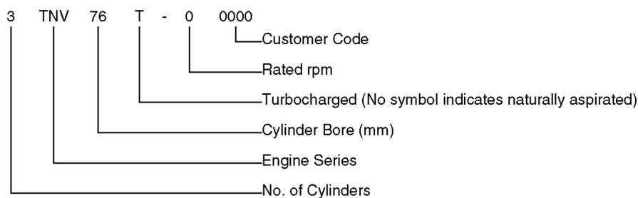
When ordering parts or making an inquiry about the engine you are working on, be sure to include the complete model and serial numbers as shown on the engine nameplate. See *Location of Labels on page 4-4*.
