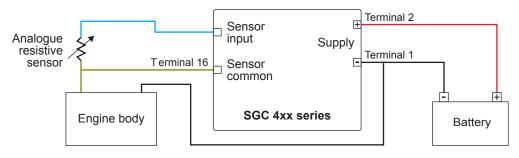
\*SCP connections for Analogue input 2 used as Fuel level sensor with the reference configured as Battery Negative
