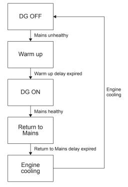
AMF mode is activated when Site monitoring, Cyclic and Exercise modes are disabled, and Mains monitoring is enabled.
