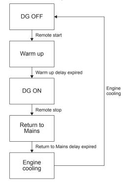
To use the Remote start/stop mode, configure one of the digital input as Remote start/stop (Latched type input) and set the controller to Auto mode. Disable Site monitoring and Cyclic mode.
