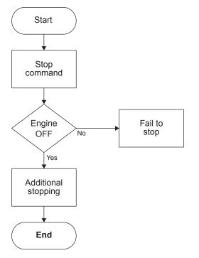
When the controller receives the Stop command, it goes to the Stop state, starts the Stop action time and activates the Stop solenoid output.
