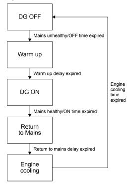
Cyclic mode is used to run the genset for a pre-specified time for a maximum cycle of 12 hours. The genset running time is configurable.
