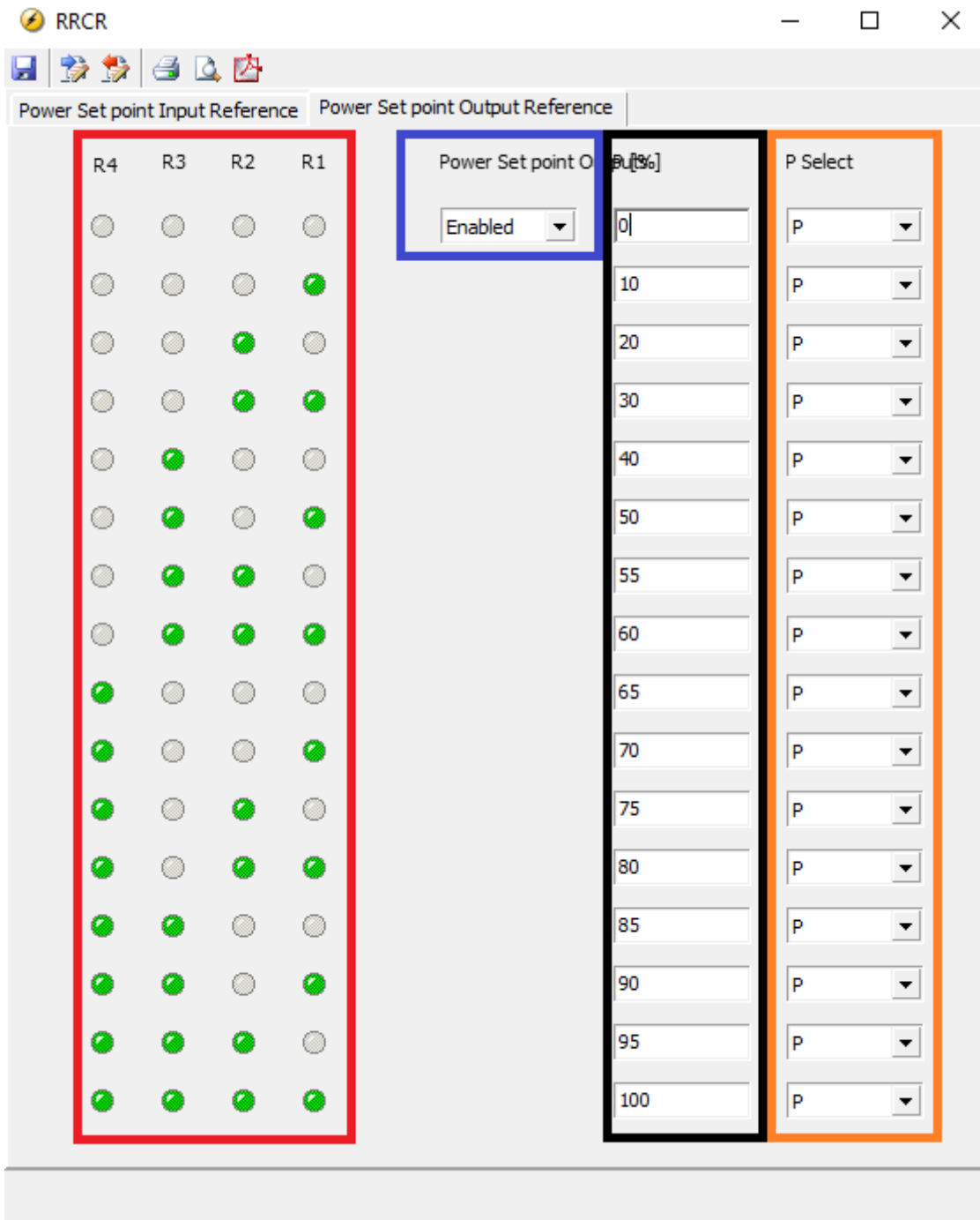
Figure 6.5 Example of power set point outputs for RRCR
