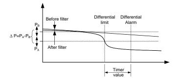
Six differential measurements between two analogue input values can be configured, dependent on the unit options.
