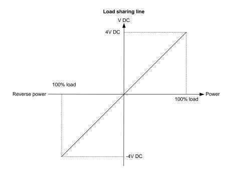
The characteristics of the reactive load sharing line are equivalent.
