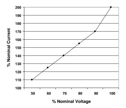
This means that if the voltage drops, the over-current set point will also drop.
