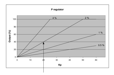
In this example we have a 2 % regulation deviation and an adjusted value of the Kp = 20. The calculated regulator value of the unit is 40 %. Now the pulse length can be calculated with a period time = 2500 ms:
