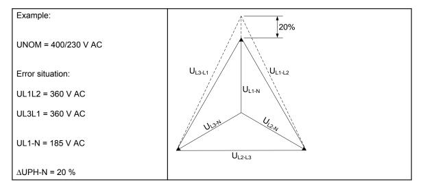
Phase-neutral or phase-phase: Both the generator protections and the busbar protections use the selected voltage.
