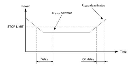
The load-dependent start relay reacts based on the power measurement of the controller together with the breaker closed feedback.
