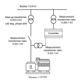
When used for synchronising, the controller uses the ratio of the nominal voltages of the generator and the busbar when calculating the AVR set point and the voltage synchronising window (dUMAX).
