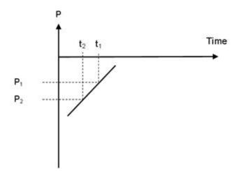
The diagram above shows that when the reverse power increases from P1 to P2, the delay will also be shorter.
