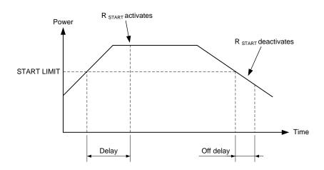
The load-dependent start relay reacts based on the power measurement of the controller together with the breaker closed feedback.
