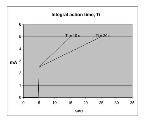
As seen on the drawing, the output reaches 5 mA twice as fast at a Ti setting of 10 s than with a setting of 20 s.
