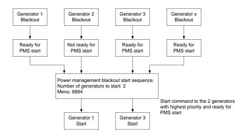
The blackout start sequence will activate the automatic start sequence, starting the generators with the highest priority and the second highest start priority (if selected), which at the same time are "ready for PMS start".
