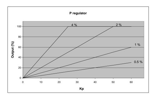
In this example, we have a 2 percent regulation deviation and an adjusted value of the Kp = 20. The calculated regulator value of the unit is 40 %. Now the pulse length can be calculated with a period time = 2500 ms:
