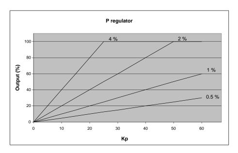
The diagram shows how the output of the P regulator depends on the Kp setting. The change of the output at a given Kp setting will be doubled, if the regulation deviation doubles.
