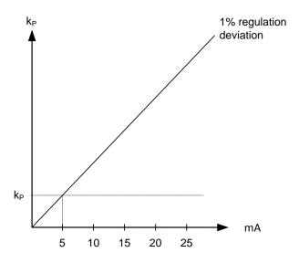
A 1 % regulation deviation occurs. With the Kp setting adjusted, the deviation causes the output to change 5 mA. The table shows that the output of the PPM-3 changes relatively much, if the maximum speed range is low.
