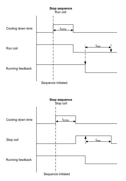
The stop sequence will be activated, if a stop command is given. The stop sequence includes the cooling down time if the stop is a normal or controlled stop.
