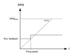
The diagram illustrates how the digital running feedback (terminal 117) is activated, when the engine has reached its firing speed.
