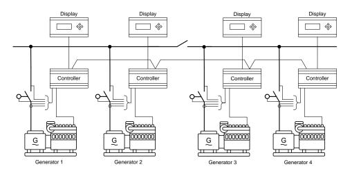
Generators can be added on both sides of the bus tie breaker.
