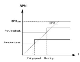
The diagram illustrates how the remove starter input is activated, when the engine has reached its firing speed. At the running speed, the digital running feedback is activated.
