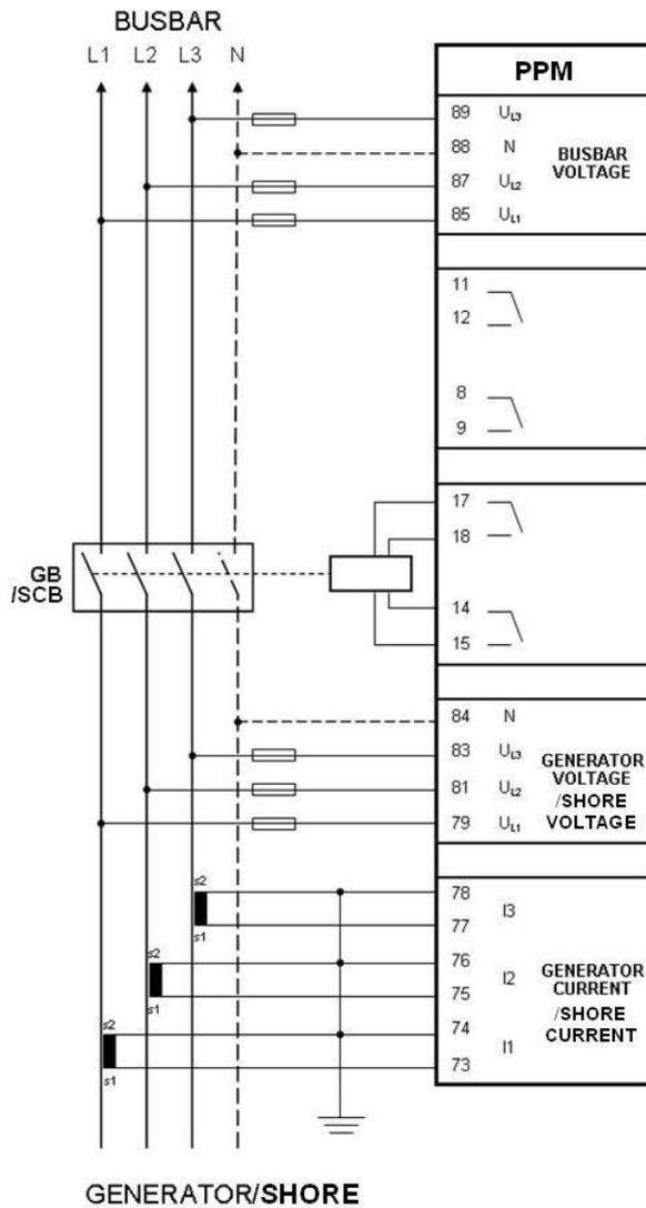
**i** The neutral line (N) connection is not necessary for correct measurement. 3-phase without neutral is also possible. The current transformer ground connection can be on s1 or s2 connection, whichever is preferred. Fuses: 2 A slow-blow.
