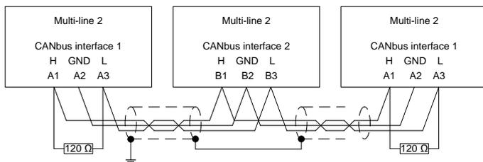
**i** CAN interface 1 and 2 can be used at the same time (redundancy) or a mix can be used, as illustrated above.
