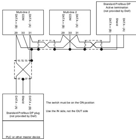
**i** Connect shield to ground at one end only. Shield ends must be insulated with tape or insulation tubing.
