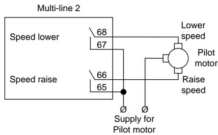
In order to extend the lifetime of the internal relays and prevent unwanted switching noise, it is recommended to use free wheel diodes (1N4007), if a DC voltage is used for the regulation. If an AC voltage is used for the regulation, it is recommended to use a varistor. The diode/varistor must be placed across the terminals of the pilot motor/external regulation relay coil.
