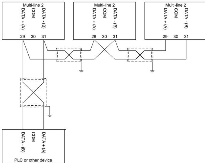
**i** Connect shield to ground at one end only. Shield ends must be insulated with tape or insulation tubing.
