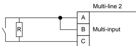
**i** The resistor value should be  $270 \Omega \pm 10\%$ .
