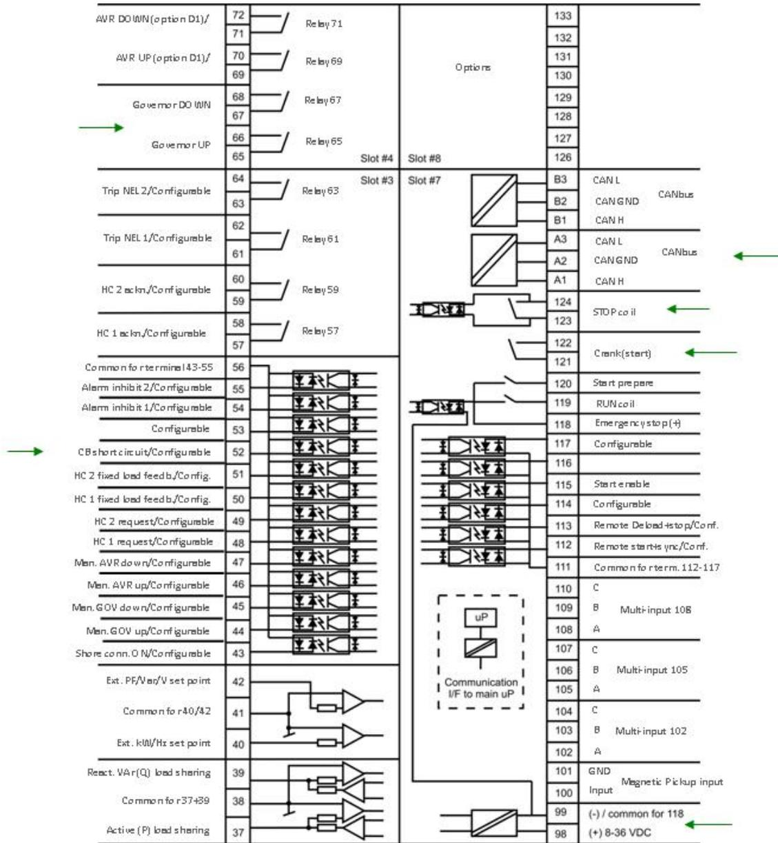
**i** Multi-inputs 102, 105 and 108 are as default set to digital input with wire break detection.
