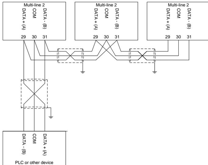
**!** Connect shield to ground at one end only. Shield ends must be insulated with tape or insulation tubing.
