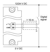
Figure 4.18 Example: Closed contact for compliance with EN60255-26
