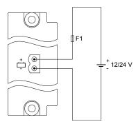
Figure 4.57 Incorrect wiring of the power supply
