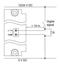
Figure 4.24 Example: Twisted wire for compliance with EN60255-26
