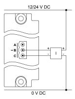
Figure 4.39 Connection of a passive transducer
