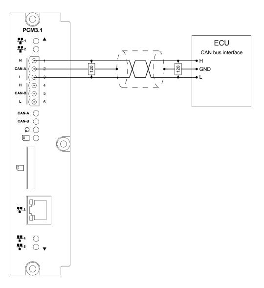
Use 120  $\Omega$  (Ohm) shielded twisted pair cable. Terminating resistors at the ends of the cable must be 120  $\Omega$  (Ohm).
