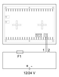
Figure 4.97 Incorrect wiring of the power supply
