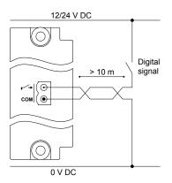
Figure 4.25 Example: Shielded wire for compliance with EN60255-26
