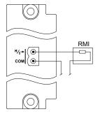
Figure 4.74 Connection of a 2-wire resistance measurement input (RMI)
