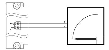
DEIF recommends using instruments from the DEIF DQ moving coil instrument series. See <a href="http://www.deif.com">http://www.deif.com</a> for more information.
