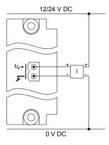
The following diagram shows the connection of a passive transducer.
