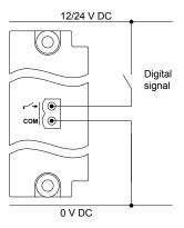
Figure 4.12 Example: Digital input wiring (common = 12 or 24 V)
