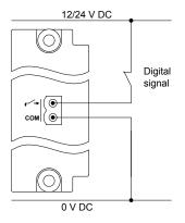
Figure 4.22 Example: Digital input wiring for safety functions (common = 12 or 24 V)
