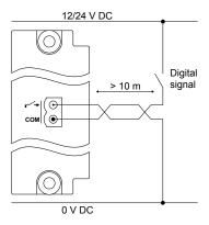
Figure 4.86 Example: Shielded wire for compliance with EN60255-26
