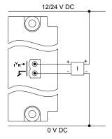
Figure 4.30 Connection of a passive transducer
