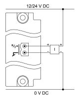
Figure 4.69 Connection of a passive transducer
