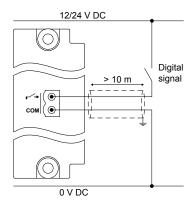
Figure 4.67 Example: Closed contact for compliance with EN60255-26
