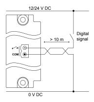
Figure 4.54 Example: Shielded wire for compliance with EN60255-26
