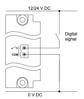
Figure 4.49 Example: Digital input wiring (common = 12 or 24 V)
