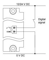
Figure 4.14 Example: Digital input wiring for safety functions (common = 12 or 24 V)
