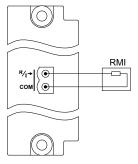
Figure 4.75 Connection of a dry contact with cable supervision
