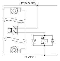
Use the following formula to calculate the maximum resistor size (in ohms):
