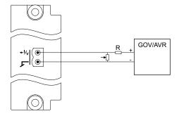
Typical value for the resistor is 2.5 k $\Omega$ , while the potentiometer is 5 k $\Omega$ .
