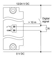
Figure 4.53 Example: Twisted wire for compliance with EN60255-26
