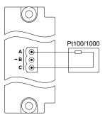
Figure 4.41 Connection of a 3-wire Pt100/1000 sensor
