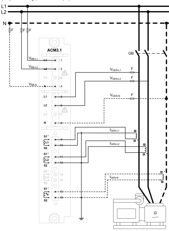
For split-phase, the waveforms are offset by a half-cycle (180  $^{\circ}$ ) from the neutral wire. Split-phase is also called L1-N-L2, or single-phase in the USA.
