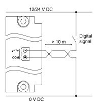
Figure 4.17 Example: Shielded wire for compliance with EN60255-26
