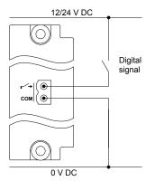
Figure 4.61 Example: Digital input wiring (common = 12 or 24 V)
