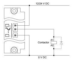
**NOTE** You can install a diode ( ) to reduce electromagnetic interference.
