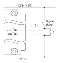
Figure 4.85 Example: Twisted wire for compliance with EN60255-26
