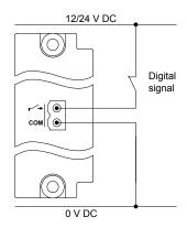
Figure 4.63 Example: Digital input wiring for safety functions (common = 12 or 24 V)
