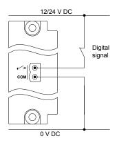
Figure 4.51 Example: Digital input wiring for safety functions (common = 12 or 24 V)
