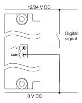
Figure 4.20 Example: Digital input wiring (common = 12 or 24 V)
