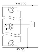
The two analogue inputs on GAM3.1 are galvanically connected. You therefore cannot use the analogue inputs on GAM3.1 in series with each other, for example, if you wanted a backup measurement. If you need two analogue inputs in series, you can use an analogue input on another module in series with an analogue input on GAM3.1, since the modules are galvanically isolated from each other.
