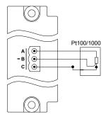
Figure 4.42 Connection of a 4-wire Pt100/1000 sensor
