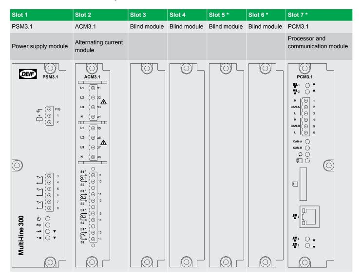
NOTE \* Alternatively, use a 4-slot rack (R4.1). Slots 5, 6 and 7 are only available in a 7-slot rack (R7.1).
