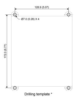
NOTE The drilling template drawings are meant as guidelines. Use the dimensions given to create your drilling template.
