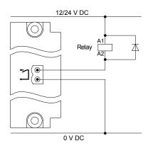
Install a freewheeling diode ( ) to prevent a sudden voltage spike across the inductive load when the voltage source is removed.
