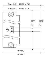
We recommend a 2 A slow blow fuse for F1 and F2, and that the diodes are rated 50 V or higher.
