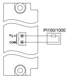
Figure 4.71 Connection of a 3-wire Pt100/1000 sensor
