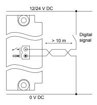
Figure 4.66 Example: Shielded wire for compliance with EN60255-26
