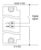
Figure 4.81 Example: Digital input wiring (common = 12 or 24 V)
