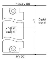
Figure 4.83 Example: Digital input wiring for safety functions (common = 12 or 24 V)
