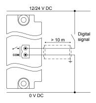
Figure 4.87 Example: Closed contact for compliance with EN60255-26
