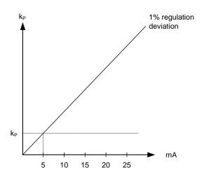
A 1% regulation deviation occurs. With the Kp setting adjusted, the deviation causes the output to change 5 mA. The table shows that the output will change relatively much, if the maximum speed range is low.
