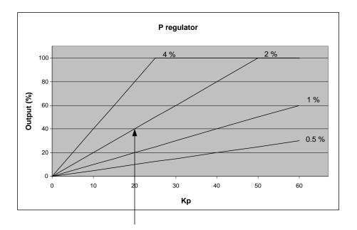
The signal length is calculated compared to the adjusted period time. In the drawing below, the effect of the proportional regulator is indicated.
