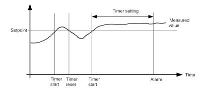
When the timer runs out, the output is activated.
