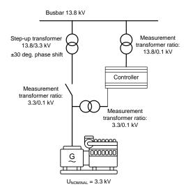
When used for synchronising, the GPU-3 uses the ratio of the nominal voltages of the generator and the busbar when calculating the AVR setpoint and the voltage synchronising window (dU<sub>MAX</sub>).
