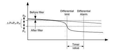
Six different differential measurements between two analogue input values can be configured, dependent on the unit options.
