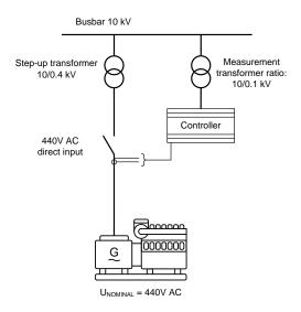
The current measurement point must be placed on the generator side of the step-up transformer.
