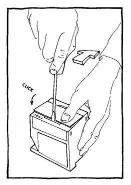
Press with a screwdriver as indicated by the arrow and simultaneously press the front panel down with your thumb. It is recommended that one side of the front panel snaps into place before the other.
