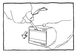
The front panel is removed by means of a screwdriver. The front panel may be loosened in the right side first and is then totally demounted by moving the screwdriver towards left.
