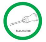
Tighten the screws only by hand and with a maximum at 0.5 nM torque to avoid overtighten the screws.
