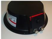
The transport lock (bright red plastic) is mounted to prevent the pointers from being damaged under heavy vibration and shock (transportation). The transport lock must be removed before connecting the indicator!
