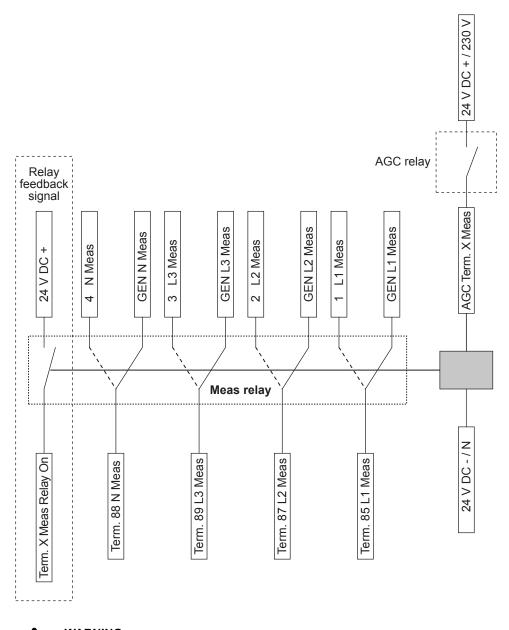
High voltages may be present between the poles on the relay (mains/generator).
