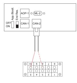
The DU-2 CAN bus communication is intended for DEIF use only and cannot be connected to other CAN bus systems.
