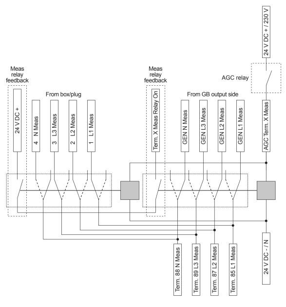
High voltages may be present between the poles on the relay (mains/generator).
