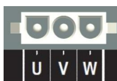
Figure 1 : Alternator voltage sensing
