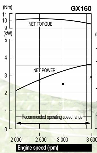
The power rating of the engine indicated in this document is the net power tested on a production engine for the engine model and measured in accordance with SAE J1349 at a specified rpm. Mass production engines may vary from this value. Actual power output for the engine installed in the final machine will vary depending on numerous factors, including the operating speed of the engine in application, environmental conditions, maintenance, and other variables.
